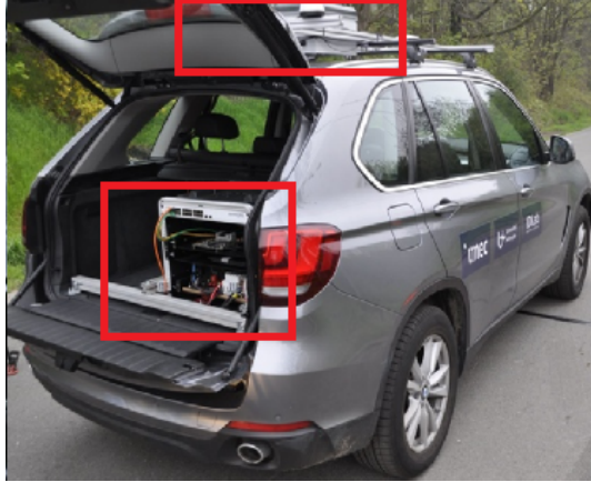
(b) The OBU Roof Unit placed on the vehicle roof and the OBU Car Unit placed inside of vehicle.
