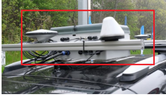
(a) The OBU Roof Unit mounted on the roof together with the GNSS antennas.
